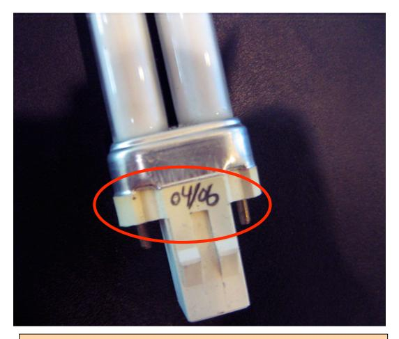
Exhibit 2 shows a CFL bulb that was removed on March 05, 2009. This picture also indicates when this bulb was installed, a policy the maintenance staff implemented to track the life of these bulbs. This particular bulb had a lifetime of close to 3 years demonstrating the efficiency of these bulbs.
